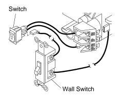
Figure 17 - Connecting the Wire Terminals
